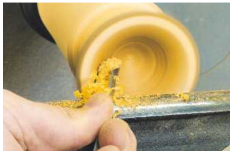
▲ Pic.3 Hollow the bowl using a series of pull cuts; cutting from the centre to the outside means you're cutting with the grain and is the best way to remove the bulk of the material
